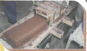
Animal Feed Block Making Machine: About 40 feed blocks per hr can be prepared with this unit. Different feed ingredients are metered individually in the pre-decided proportion and mixed to make the feed block.
